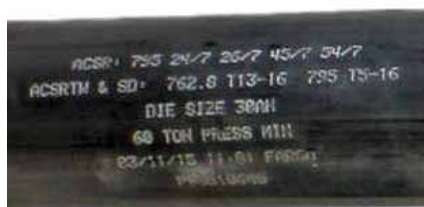
Above: close up of marking on Fargo splice requiring 14SH die index.
